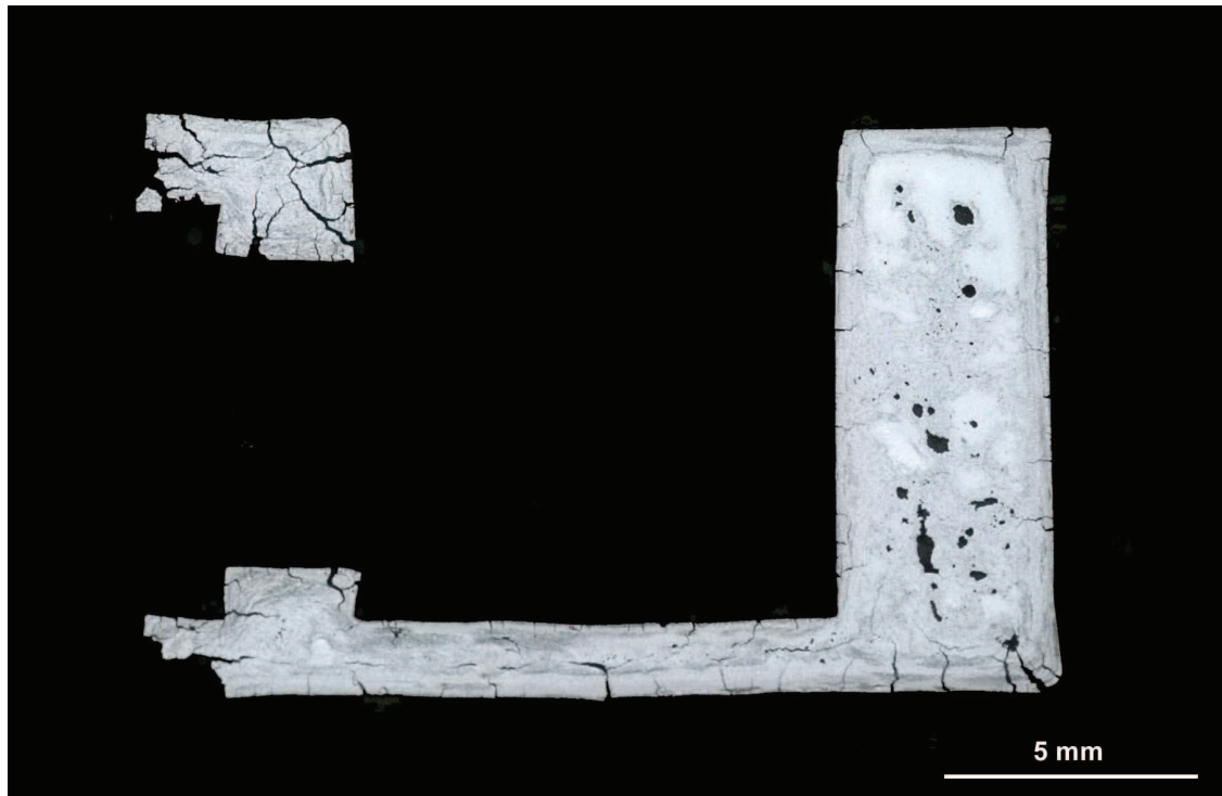
Fig. 5 Metallographic overviews of the cracking in the wheel (top) and block (bottom). Note the porosity also
