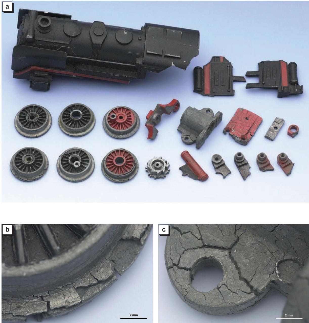
Fig. 1 Severe corrosion-induced cracking in a zinc-aluminium die cast model locomotive, vintage 1946-1947. The details in figures 1b and 1c show part of a wheel and a block fitting
