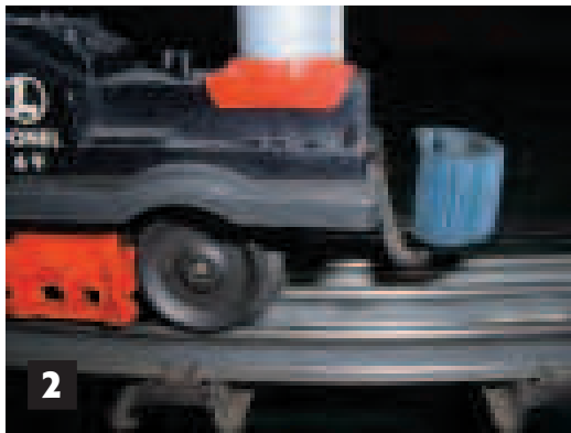
Photo No.2 shows the die cast platform support and the U reversing plate on the prototype.
