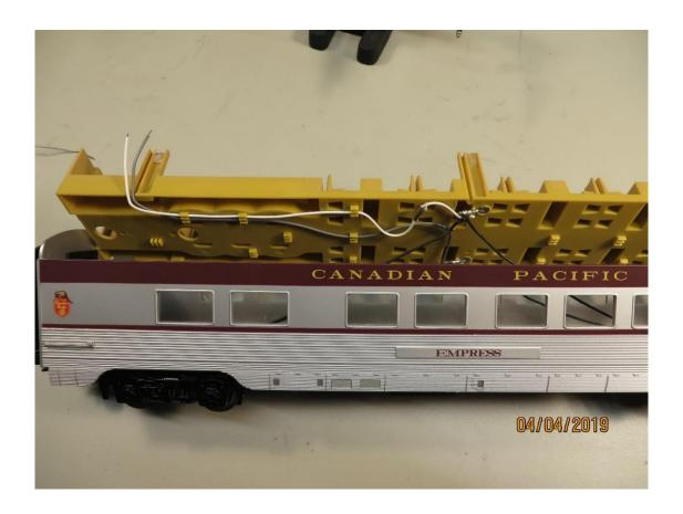
3. Select a suitable location for the lighting module, usually in an end vestibule, washroom, service corridor, or other inconspicuous area. Strip out all the old lighting but save one pair of track power wires long enough to reach the module location. These wires will be soldered to the AC input of the module later.
