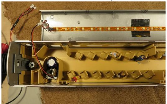
Note the common parallel hot wire between the power pickup rollers should remain intact for power to the module as detailed later.
