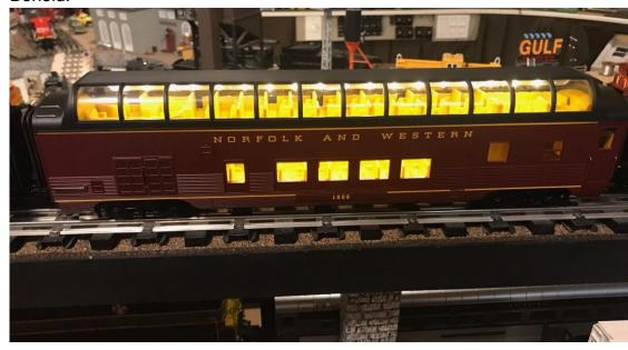
9. A typical observation car will have red side marker bezels and a taillight bezel, either red or white. These can be lit by using 3 flat top 3mm white leds wired in series with a suitable 220-330 ohm resistor. This circuit can be soldered to a convenient set of copper pads on the main led strip for power. Then bend the led leads with pliers to align the led face right at the inboard end of each bezel.
