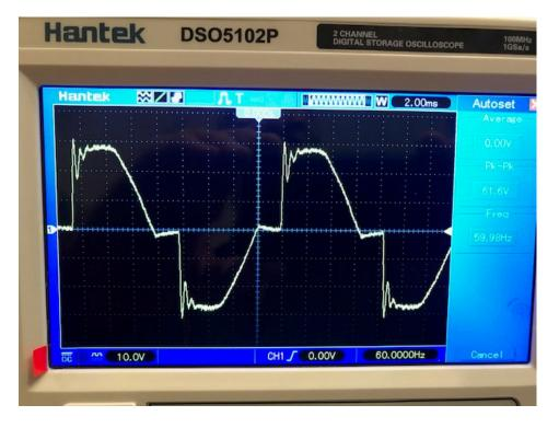
Here is the pattern for 18 V output. 61 volts P-P
