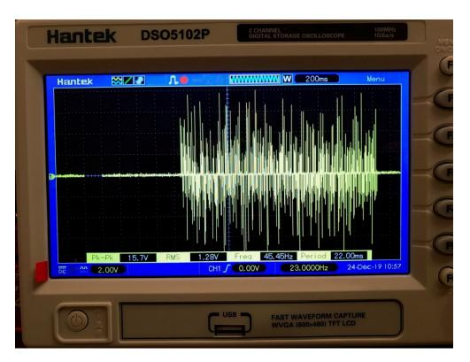
TIU Startup Burst; Vert set to 2 V/D; Hor set to 200 ms/s. Hash pattern ~15 V P-P lasting ~ 3 secs. Only present when TIU is powered up with NO voltage supply to the channel inputs. No idea what this is for?
