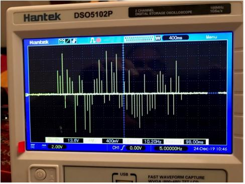
TIU V1/V2 Output Voltage Pattern. Vert set 10 V/D, Hor set 2 mv/D. 71 volts P-P. The variable outputs show a very strange "curve" output as shown below for 12 V on handheld:
