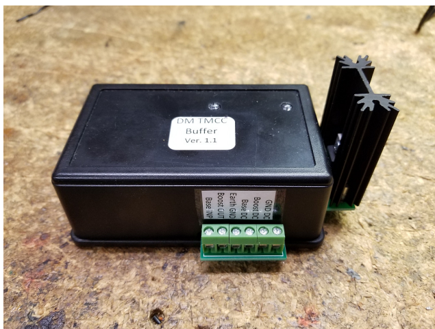
Figure 2 TMCC Buffer Power Amp
