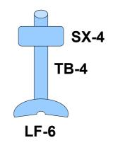
TB-8 fits inside LF-412 TB-4 fits inside TB-8 Cut off tip and drill 1/8 inch hole in LF-6 for TB-4
