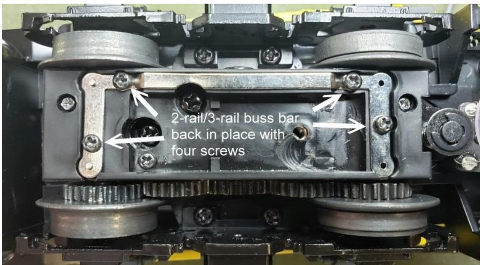
With the nubs in their new position, use the four screws to re-install the buss bar and then re-attach the center rail rollers.
