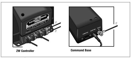
Figure 5. Command Base connection
