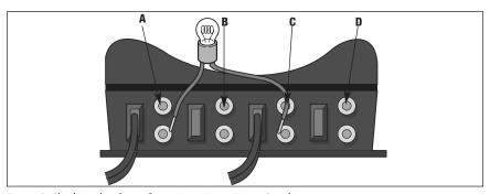
Figure 8. Checking the phase of your PowerHouse Power Supplies
