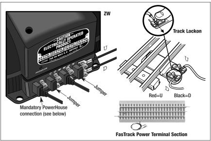
Figure 2. Lock-On connections
