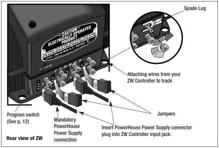
Figure 3. PowerHouse connections
