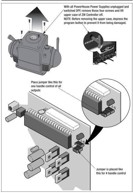
Figure 9. Setting the jumper
