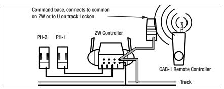
Figure 6. TrainMaster Command Control and the ZW Controller
