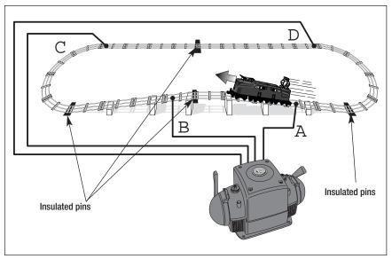
Figure 10. Control of various track blocks
