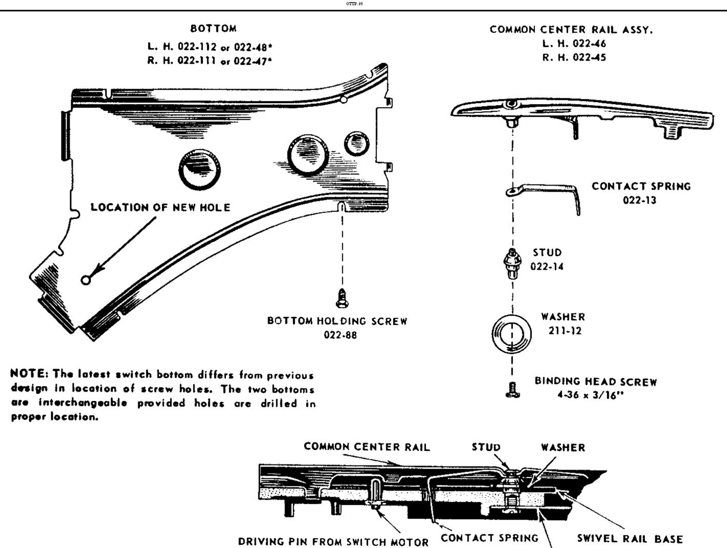
Cross-section view showing how the common center rail is assembled to the switch base. The driving pin which is shown engaged to the swivel rail is part of the motor switch assembly not shown in the illustration.
