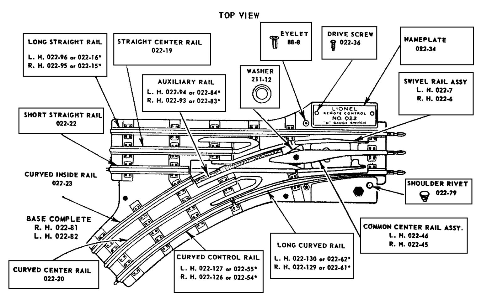
filustrations on this page show the top and bottom views of the left-hand switch base. The companion right-hand switch base is its mirror image except for the location of the steel track pins and the section which makes contact with the switch motor. In 1950 a number of changes were made to facilitate production. However, the old parts, marked by asterisks, may be used interchangeably with the new parts except as noted.
