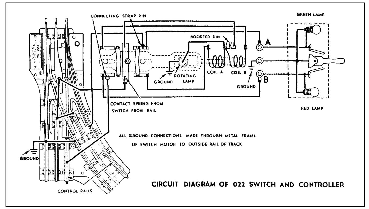
In order to prevent a train from running into an 'open' switch and thus derailing itself. No. 022 switches are provided with 'control' rails which automatically throw the switch to a correct position for the passage of the approaching train.
