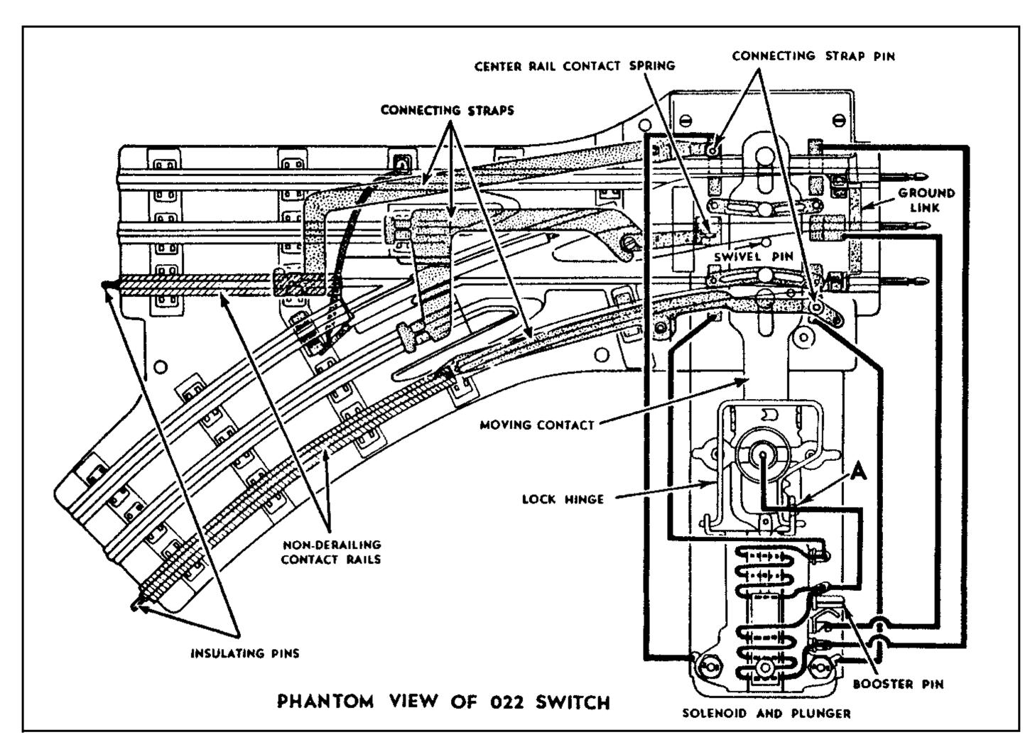
tension of the springs to see that proper contact is made at all four points of contact.
