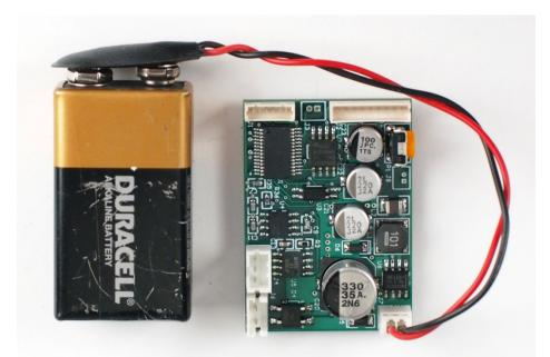
Figure 5 – Battery clip installed in RAILSOUNDS board. If operating your loco without a battery installed, cover the exposed battery clip terminals or the RAILSOUNDS board may be destroyed.
