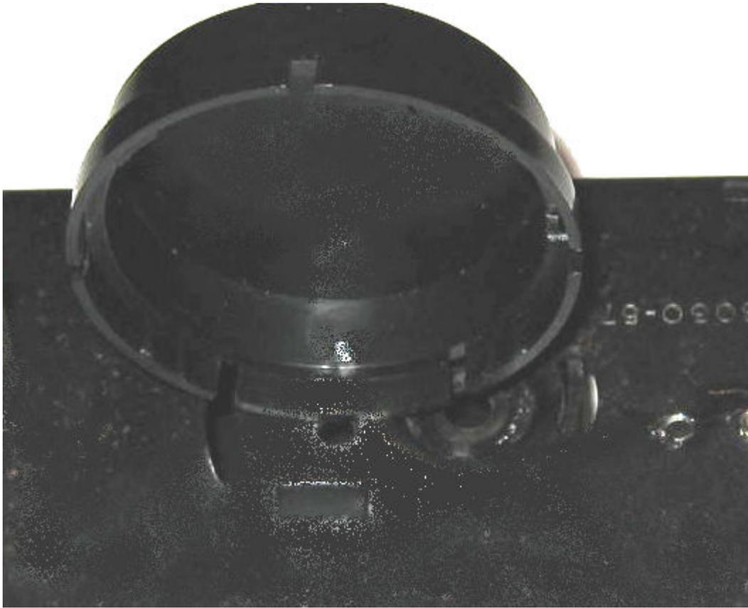
4. When the speaker is installed inside a loco, it is protected and therefore does not require the cover installed. Use one of the methods below to secure the speaker in the baffle:
