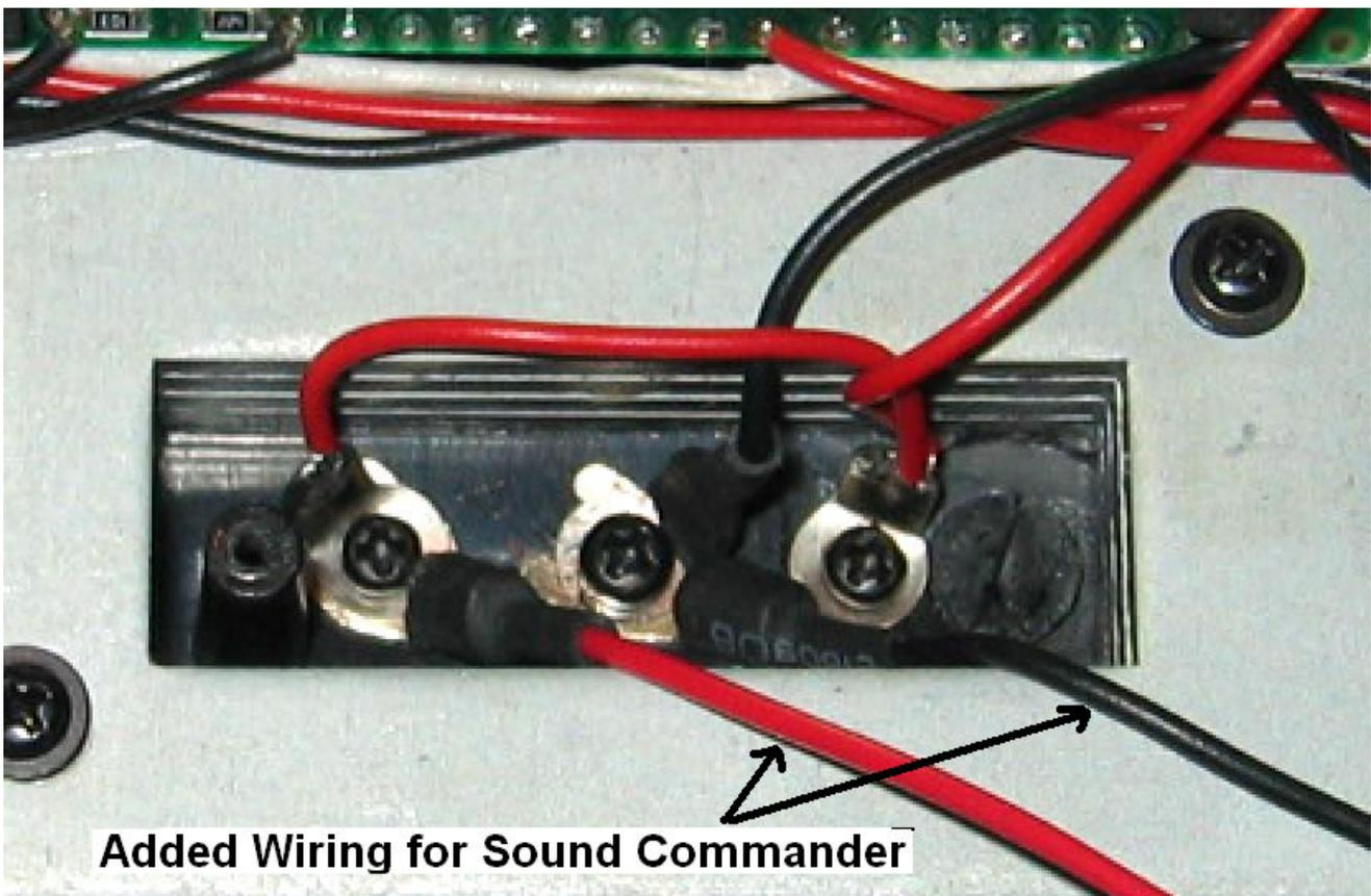
After attaching the Sound Commander 2 power cable, set the Beep power chassis aside. Proceed to “Installing the Sound Commander 2” on page 11 to finish the installation.
