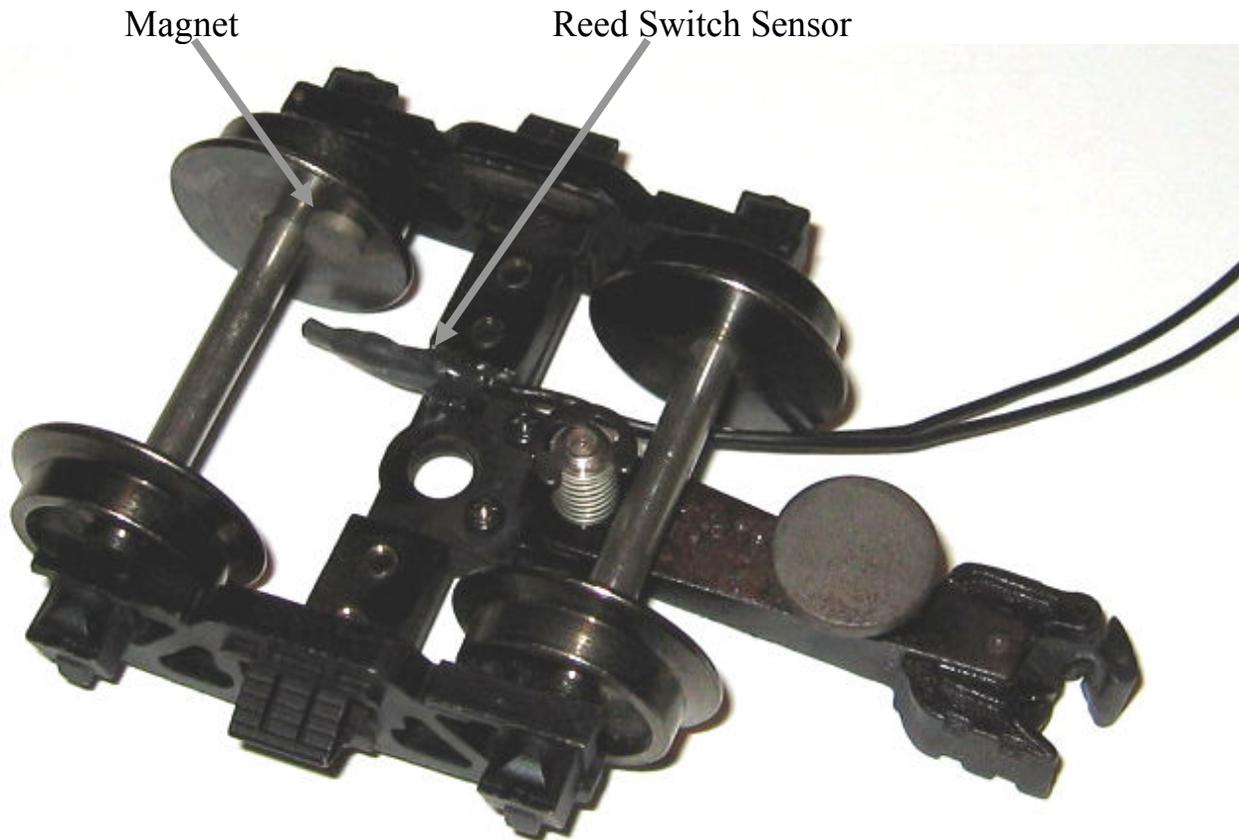
3. If needed, drill about a 1/8" hole in the tender chassis to route the leads up into the tender insides to connect to the "chuff" input on the Sound Commander 2. Do this before mounting the truck back onto the chassis. Protect any installed electronics from metal debris when drilling the hole. De-burr the hole to prevent chaffing the wires from the chuff sensor. Next reattach the truck, routing the chuff sensor wires into the tender.
