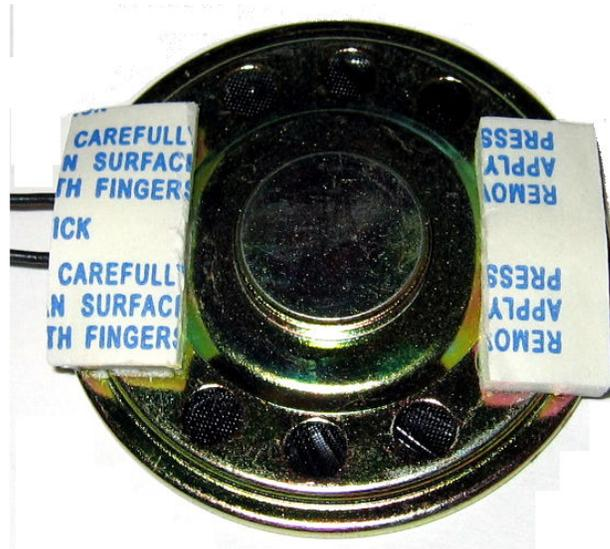
2. Remove the window treatment in the Beep’s cab shell. Install the speaker as shown. The wires are directed towards the long hood on the Beep shell. Test fit the speaker first with the double stick tape protection on. Once comfortable, fasten the speaker in permanently.
