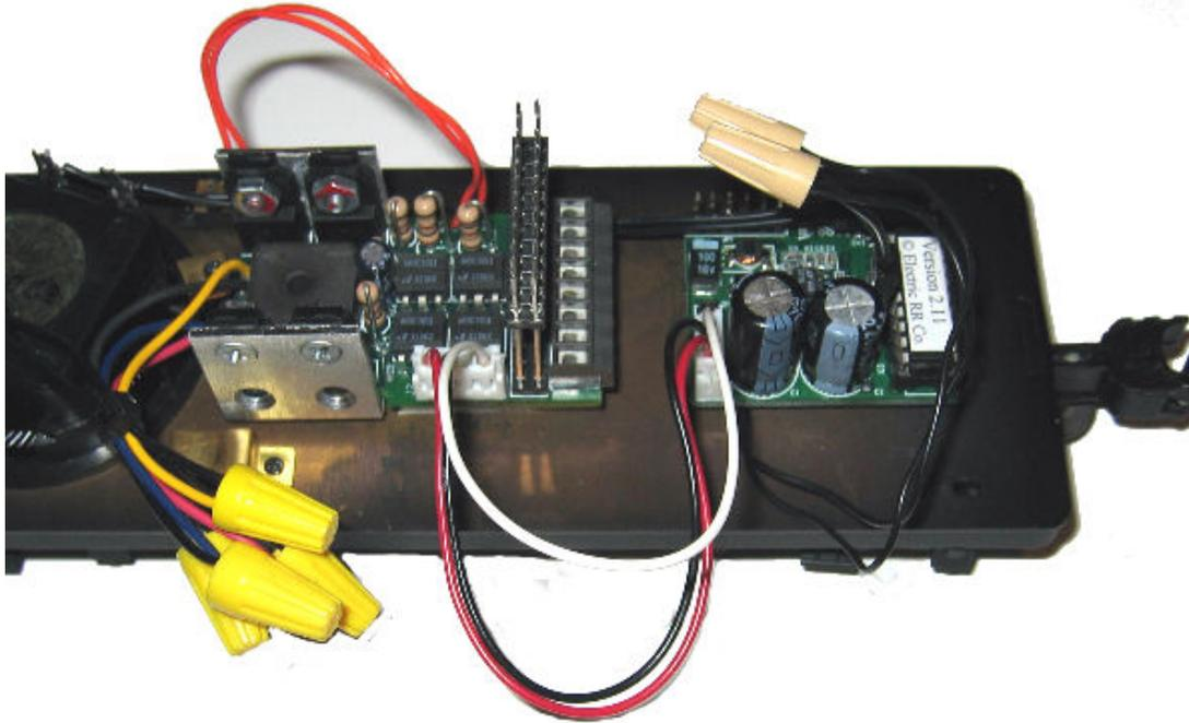
5. Use two (2) layers of a 1.0" x 1.0" piece of double stick tape on the back of the Sound Commander 2 for attachment to a metal tender chassis. Two (2) layers are used to prevent the possibility of any Sound Commander 2 backside components from shorting against the chassis. Test fit the tender shell before affixing the Sound Commander 2 permanently.
