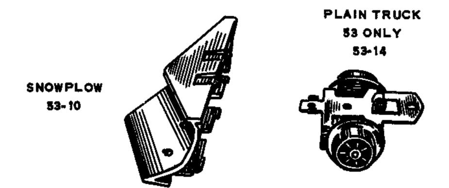
These parts are used instead of the coupler truck at the front of No. 53. The snowplow grips the end frame with four claws, one pair at the top and one pair at the bottom. To remove, squeeze one side of the plow at a time so that an upper and lower claw are pressed toward each other, and pull out.
