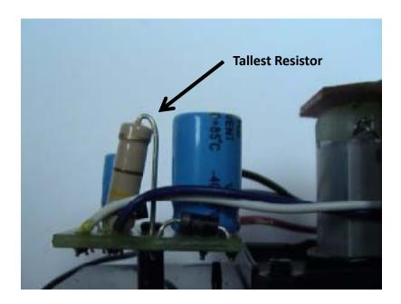
4.) Using a pair of small wire cutters cut the leg off the top of the resistor. (this leg will be used, So do not cut it off the PCB where it is soldered). The photo below illustrates how it looks when cut.
