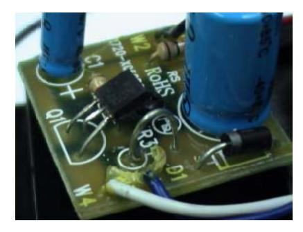
7.) Test the air whistle function now. If the whistle does not sound then the solder connection is not good and must be reheated. Once the test confirms the functionality of the whistle place the shell on the tender deck and reinstall the 4 Phillips head screws you removed in step 1.
