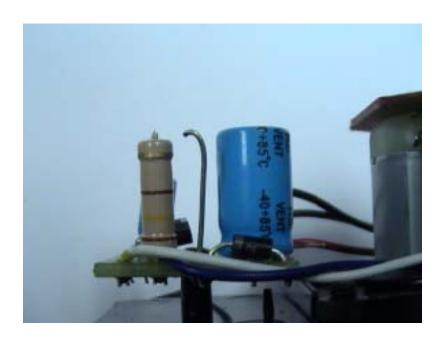
5.) Using small wire cutters cut the resistor at the bottom of its body, where it is soldered to the PCB. The PCB should look like the photo below at this point.
