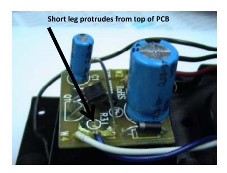
6.) Bend the long resistor leg over and solder the end to the short leg soldered at the base of the resistor. It may be necessary to scrape some of the adhesive away from the solder point, just don't break the wires off doing so! The photo below illustrates the finished repair.
