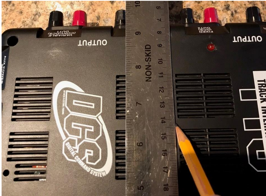
PIC 2; Draw a vertical case centerline
