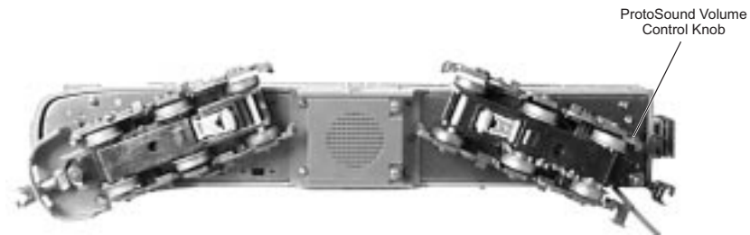
Figure 4: Adjusting The ProtoSound Volume
