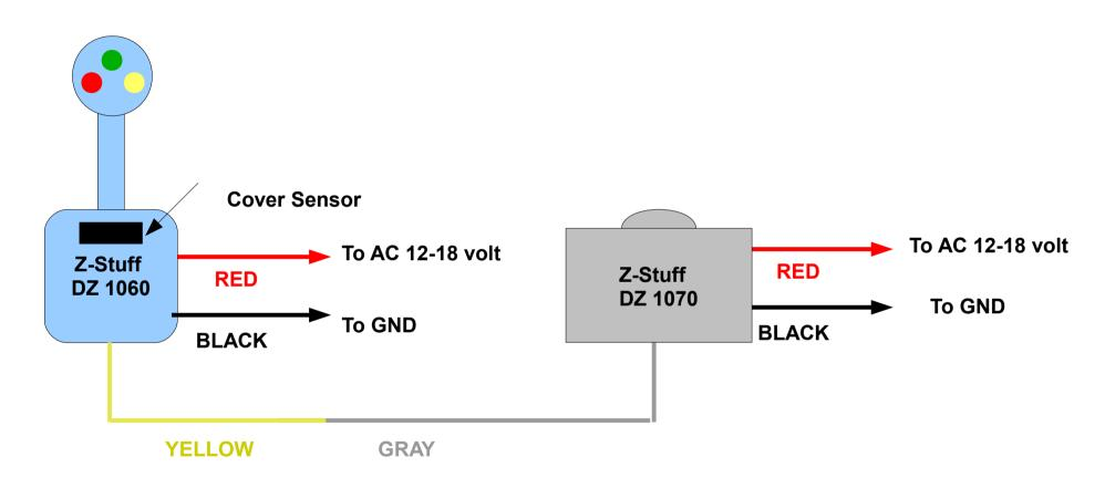
Allows signal to be remotely controlled by the 1070 sensor
