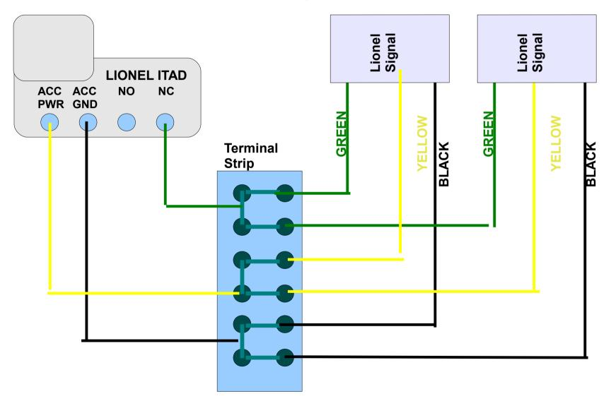
Rule of thumb – it is possible to connect multiple signals to one ITAD but not multiple ITADS to one signal
