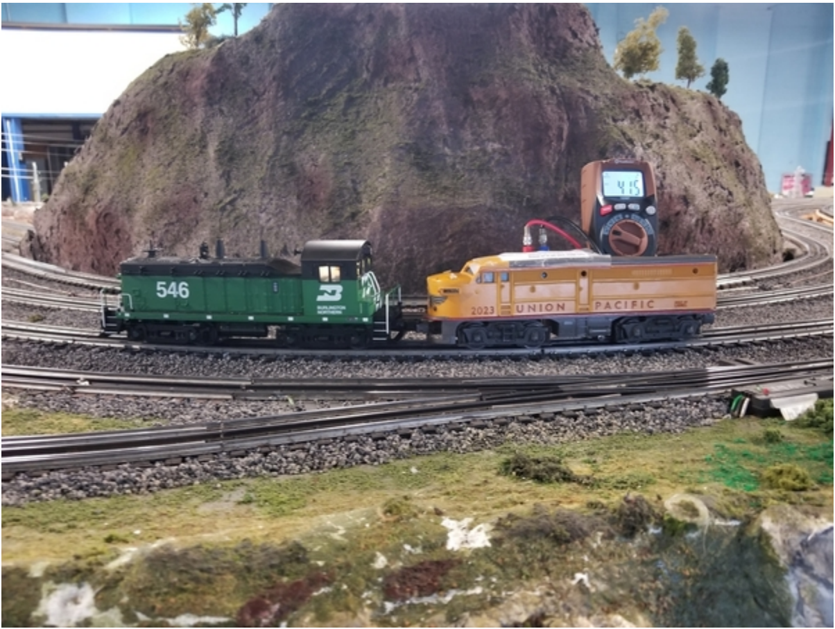
Figure 1 TMCC earth ground signal test car and bluetooth meter pulled with #546 engine
