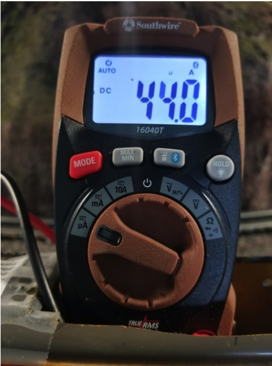
Figure 2 Southwire bluetooth meter with data recording capabilities
