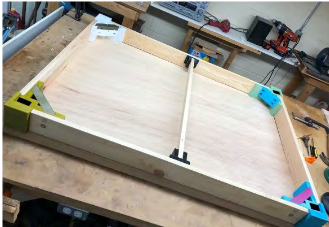
Underside of module assembled with 3D parts
