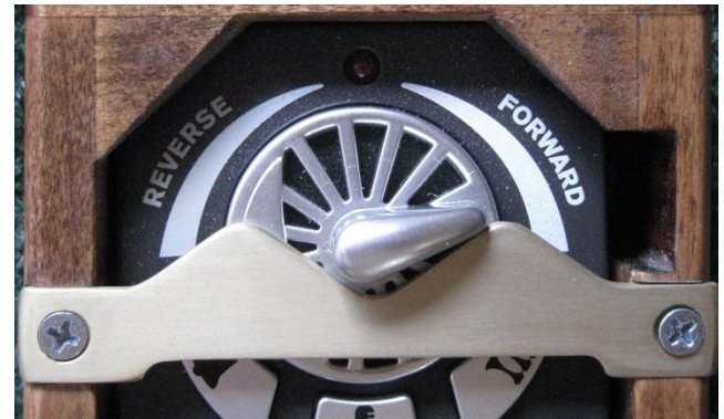
This bar permits about 150° of throttle knob rotation.
