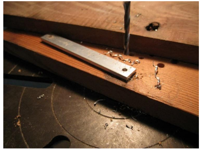
Drill through holes at each end of every piece.
