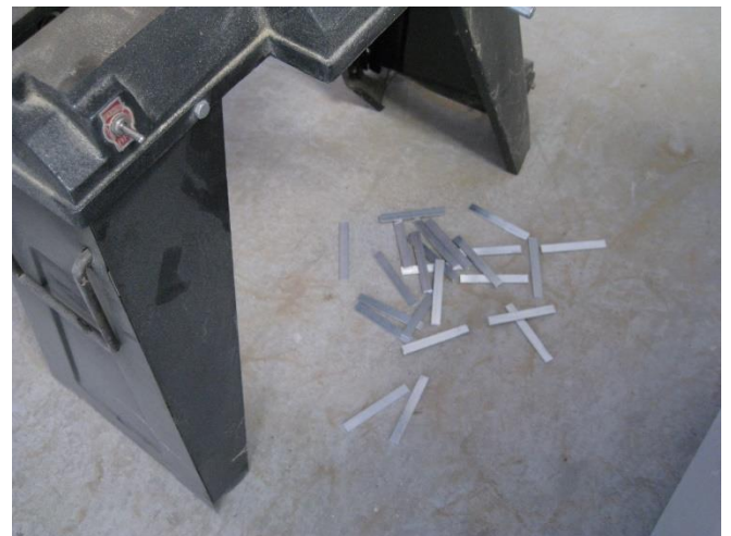
Cut enough pieces for the number of cradles being made (4 per cradle) and perhaps some extras. Some of these bars will later be cut into two filler pieces, but for ease of handling are kept as a single bar for now.
