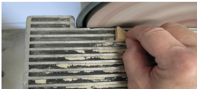
On a sander, sand the small flat on each triangular part that mounts on the side with the power switch notch.
