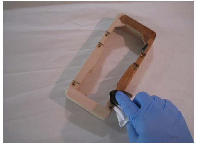
Stain all surfaces. A little stain getting on the metal inserts doesn't matter.
