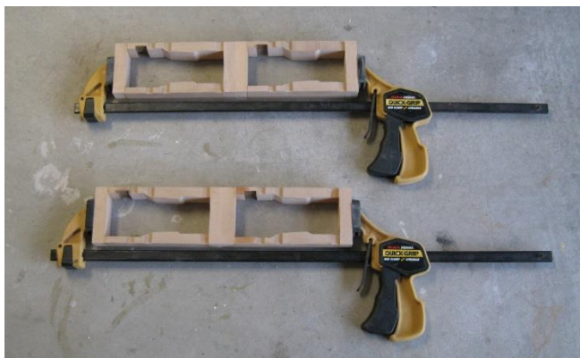
Glue the tops and bottoms to the side pieces. (Each clamp is holding two sets of parts in this example.)
