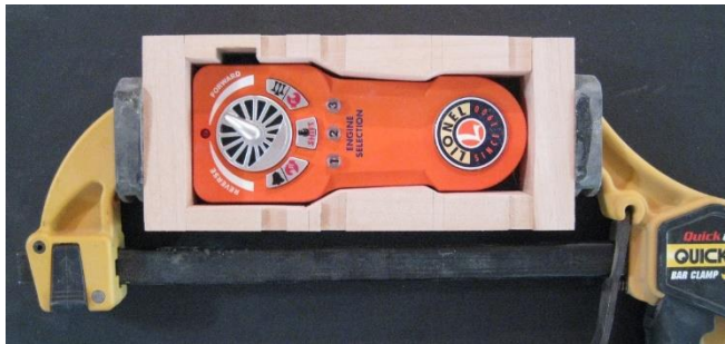
Clamp each set of parts together temporarily and make sure a controller fits without binding AND can be removed by tilting up the bottom of the controller. Correct any binding problems. Also, mark the pieces in areas that won't show to keep them together as a matched set.
