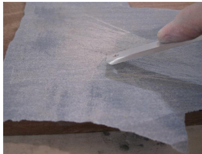
Work on the curved to remove more of the curve towards the edges while leaving most of the metal at the center intact. This will help blend it into the cradle edge. Round the corners and break all sharp edges so there is no risk of snagging a finger.
