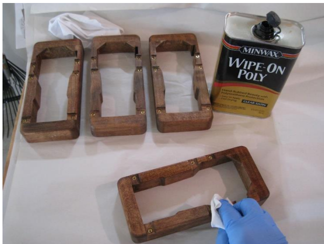
The cradles got several coats of "Wipe On Poly" by Minwax. This is very easy to use. Of course, any wood finish could be used.
