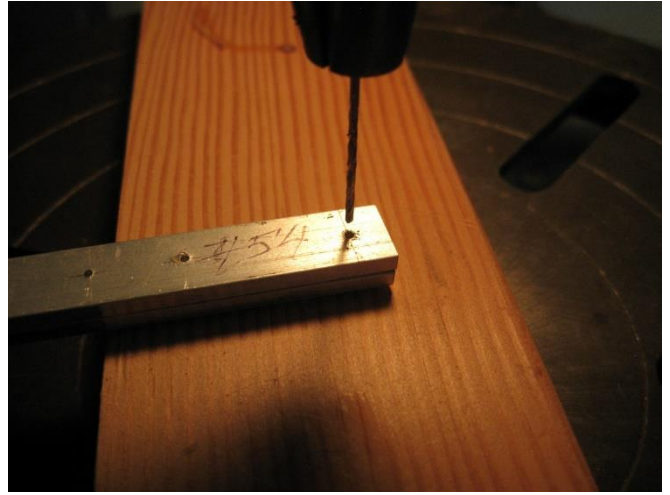
Using previously made drilling jig, drill pilot holes in all pieces.
