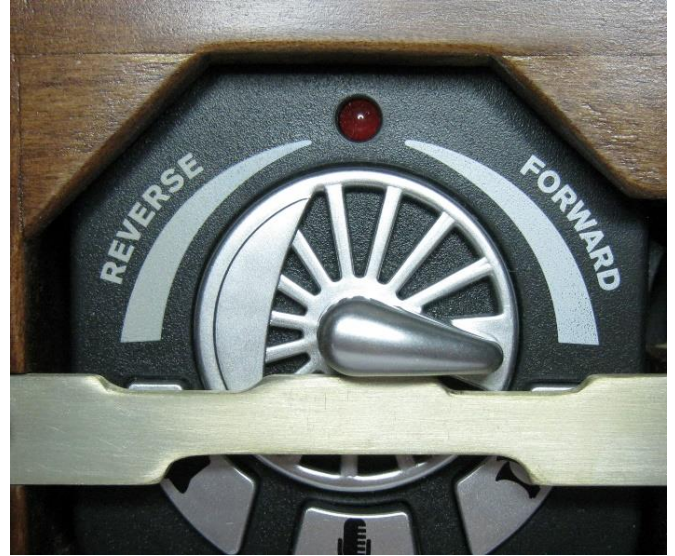
Original top bar reversed at the San Luis Obispo Railroad Museum. However, the knob protrusion is prone to rub on the bar.
