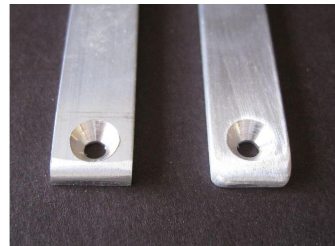
The left is from the stationary belt sander. The right is after further refining the shape.
