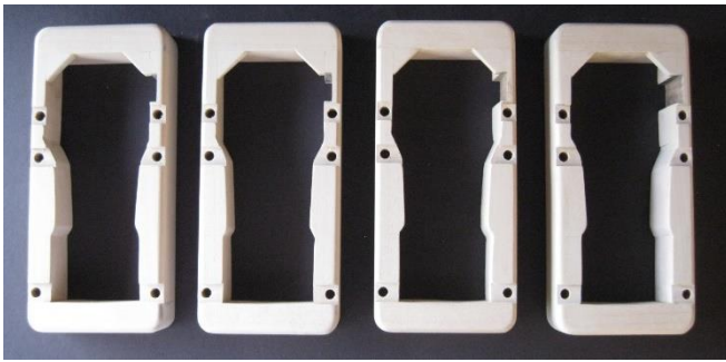
The cradles after the triangular parts glued on. Hand sand to blend them so the top surface is smooth.
