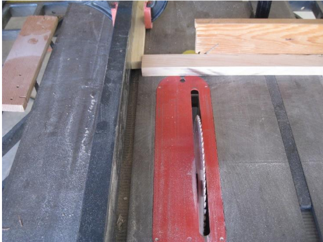
After planing to thickness and ripping to width, cut side, top, and bottom pieces to length.
