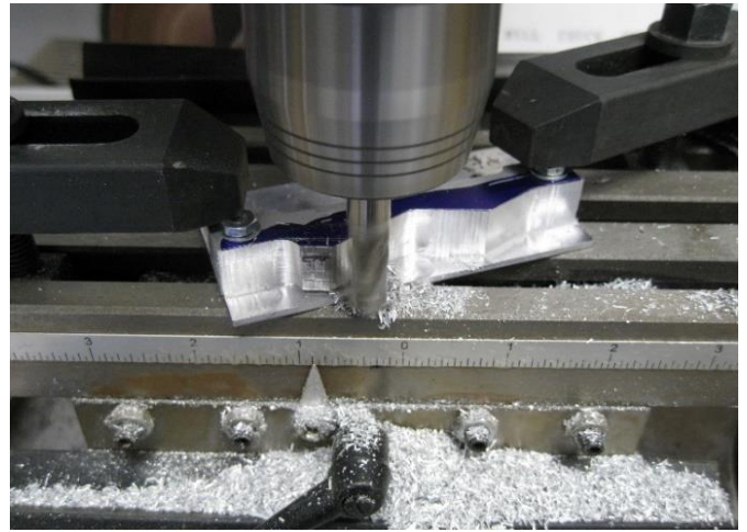
Layout dye and dimensional marking was used. Each part with angles also first had most of the metal to be removed cut off using a band saw leaving enough for finish milling. This is a stack of four 20 degree top bars being machined up to the marked lines on the top piece by eye.
