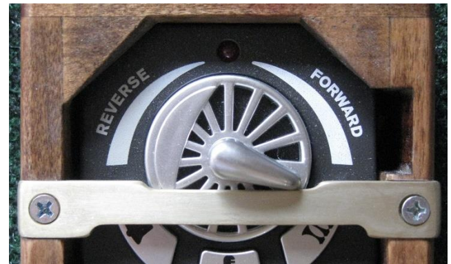
This bar permits about 220° of throttle knob rotation.
