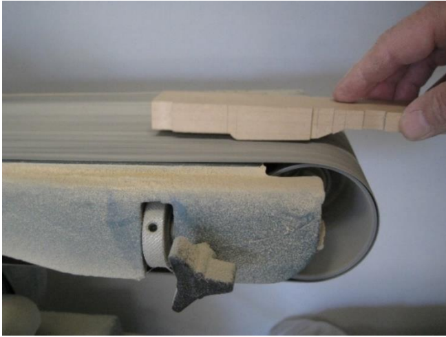
Some of the bandsaw cut edge can be sanded on a belt sander to smooth it.
