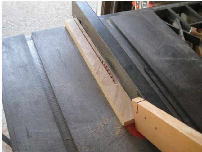
Rip some wood to the cross section for the triangular wedges.
