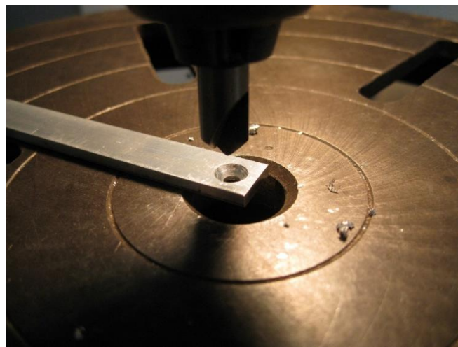
Countersink the mounting holes just enough so the screw head will be flush with the surface.
