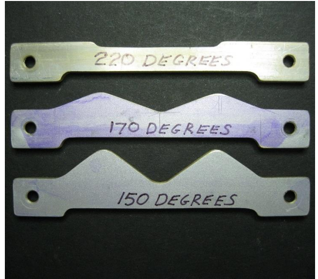
For reference, the parts were labeled simply using a permanent marker. Note that the backs of the wider pieces have no Alodine coating, and some will show layout dye staining.
