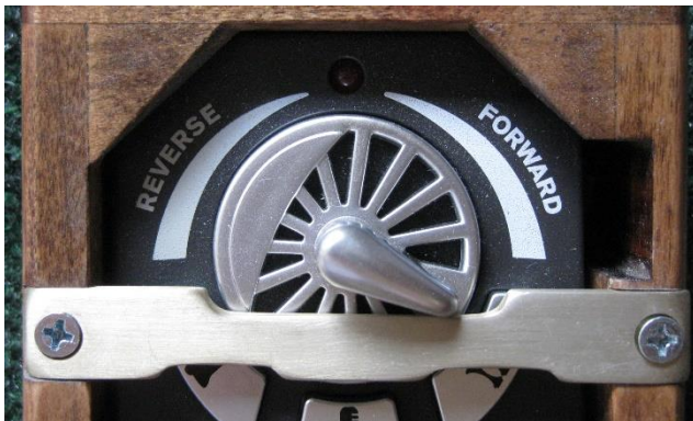
For reference, this is the original top bar that permits about 235° of throttle knob rotation. With no limiting the knob rotates about 295°.
