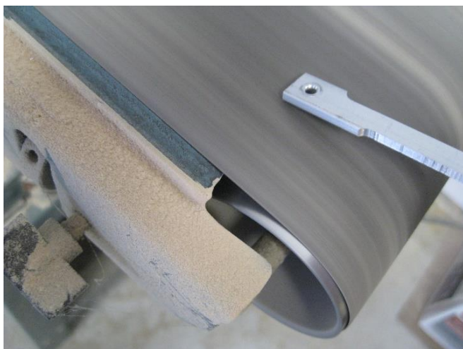
The radius at each end was done on a belt sander. Later hand work would further refine the shape of the ends.
