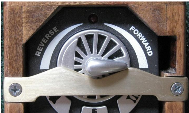
This bar permits about 170° of throttle knob rotation.
