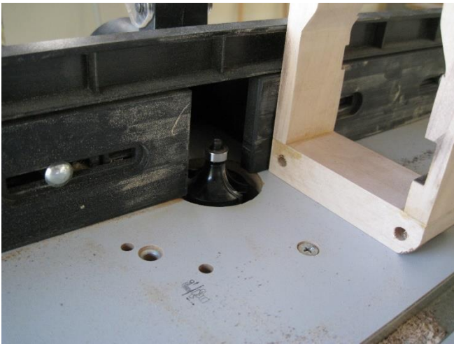
Using a router table and a ball bearing 1/2" roundover bit, route the corners.
