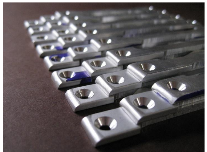
This is the batch of 8 sets of the 3 different throttle limiting top bars after the rough rounding of the ends on the belt sander.
