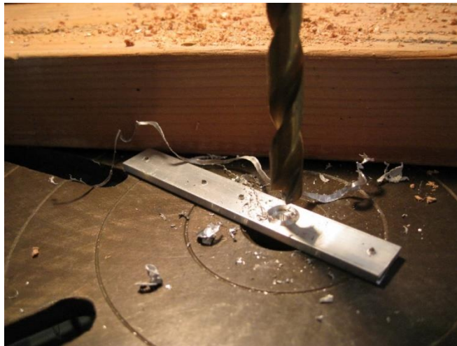
Machine counterbores in the bar optionally used with the Universal Controller. Then drill the through hole for these locations.
