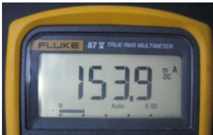
Current draw from car with incandescent lights at 18 VDC.
