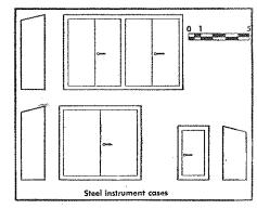
Relay and instrument cases like these are often mounted on poles, signal standards or bridges.
