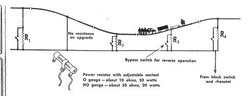
Train speed variation on grades can be controlled by running power through fixed resistors as shown here. Determine the size of resistors by trial. Note that gaps are placed where power requirements of average trains vary rather than at points where the grades actually begin and end.
