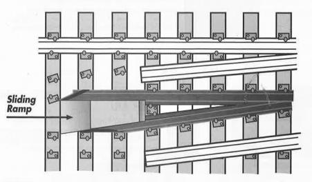
Note: The ramp is not required for magnetically activated couplers or operating cars.
