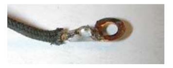
Remove the old post and insert the new one in the hole. Put the loose wire lug over the threaded stud and screw on the nut until it's tight. Make sure no other bare wires are touching the end. Replacing one of the 'U' posts is easier since it's on the top row and there are no loose wires, just the solid buss bar.
