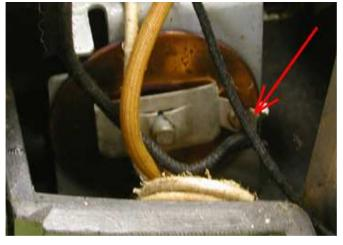
of the rectifier by slipping it under the nut and tightening it. **Note**: Just leave the old copper oxide rectifier in place; it won't interfere with the whistle control circuitry once we install the new stud rectifier.
