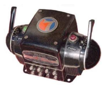
The February Tech Tip addressed how to replace the ZW power cord. This month we will show you how to replace the carbon rollers (four each) and loose or missing binding posts (eight each). Fortunately there are third party replacement parts to rectify both of these common ZW repair problems.
