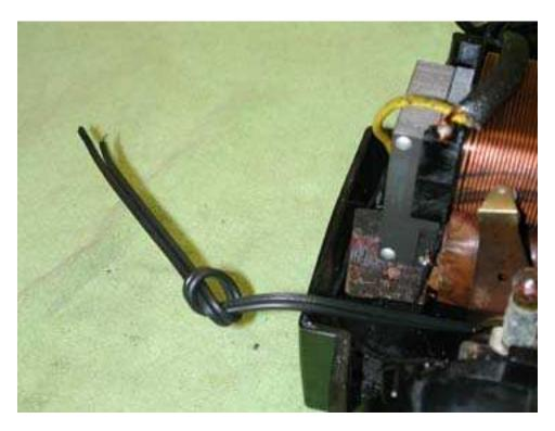
**STEP 6:** Separate the ends of the cord for two inches or so and cut one inch off one of the ends. Strip one half inch of insulation off each end, twist the ends tightly, then tin them with solder.
