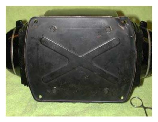
**STEP 2:** Cut the old power cord off where it enters the bottom case. Set the transformer on its bottom and warm up your soldering iron.
