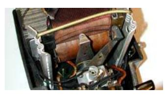
It's usually the "A" or "D" since they are the most utilized. There are two ways to replace rollers; the easy way and the hard way. The hard way entails removal of the short contact arm assembly for the "A" or "D" rollers and the easy way is to install the new rollers in place. Installing the rollers in place means you have to remove the remains of the old rollers and the rivets.
