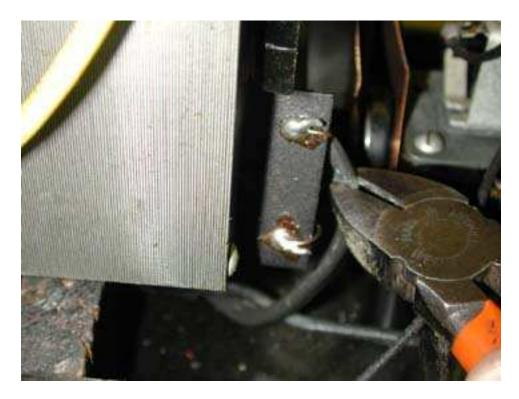
**STEP 4:** Heat up the top terminal with the soldering iron and use needle-nosed pliers to gently pull the wire free of the eyelet when the solder joint is fluid. Do the same with the bottom terminal taking care not to pull or bend the small, solid conductor primary core wires. The new power cord should be two-conductor and the same size as the old one.
