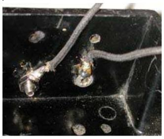
(Note: I usually remove the bottom mounting plate screws that hold the front core aluminum mounting bracket so I can slip the core mounting bracket out of the way (you'll need more room for the bottom posts) when tightening the nuts for the replacement binding posts. Place a small block of wood under the core to hold it in position while working on the posts).
