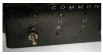
It's very common for the terminal (binding) posts to become loose, bent, or fall out altogether due to age and misuse. This isn't terrible, especially since there are bolt-on replacement posts available from you local parts dealer and they're easy to install.
