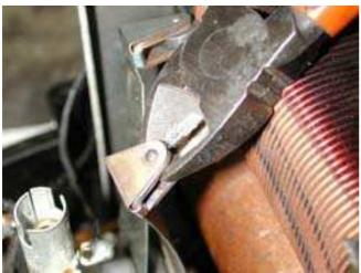
Move the "B" or "C" roller arm out of the way first. Use needle-nosed pliers to crush the bad roller and cut the rivet in the middle with diagonal cutters. Remove the two rivet halves and clean up the crushed rollers pieces from the bottom of the case. Make sure there are no loose pieces rattling around in the case.
