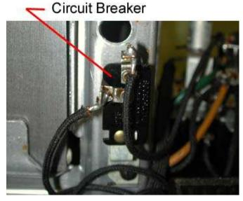
Replacing a bad breaker, fortunately, is very straight forward. If yours is the 'R' type, simply unsolder both wires and remove the mounting screw. Install the new breaker and solder the old wires back on to the terminals.
