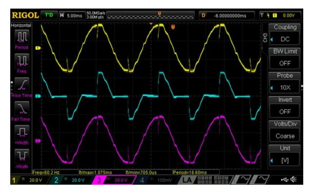
Note how the switching transients when less than full throttle whack both the fixed and variable channels, very odd. The spikes even affect the transformer output, which explains why they appear everywhere.
