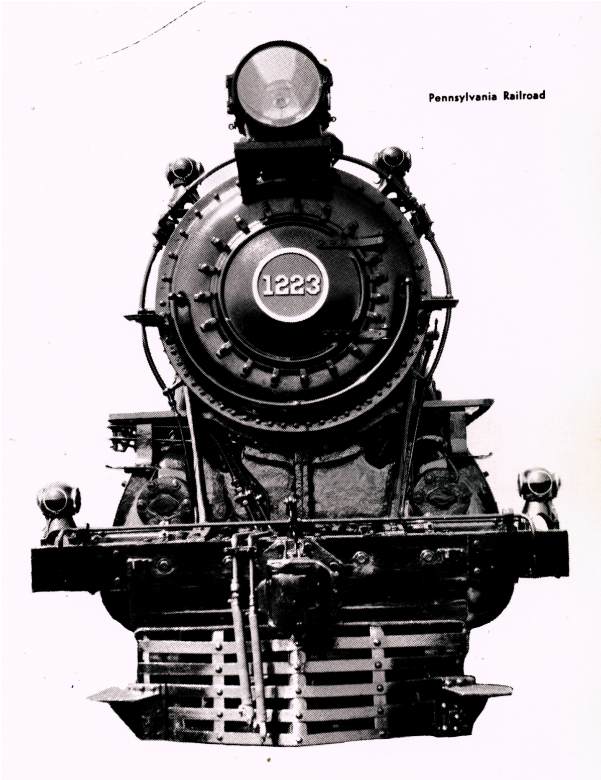
Claw Foot Style as Both Class and Marker Lights. (1922 Standard).
