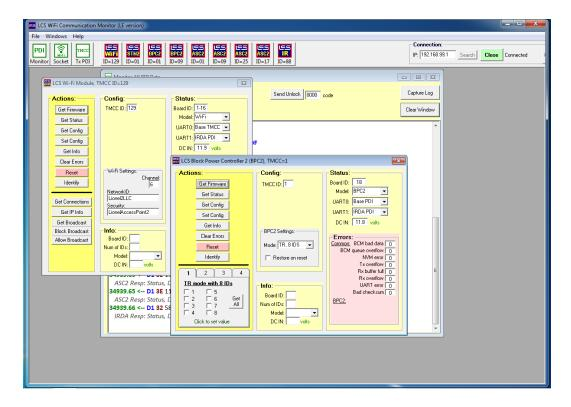
Each type of module share some basic buttons and each has details unique to just that module type. In the example above, you can see that the WiFi module and BPC 2 both have identical Action buttons.
