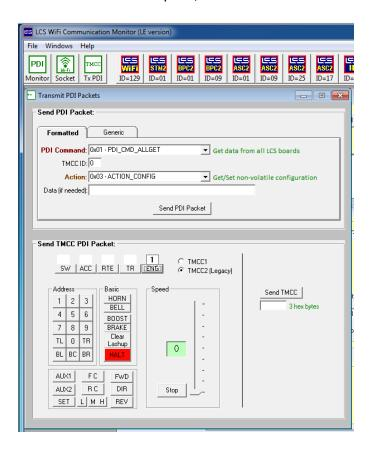
Using the Transmit TMCC PDI Packet window, you can operate engines, trains, switches, accessories and routes as though you were using a physical CAB remote. Be sure to select the appropriate style of command (TMCC1 vs. TMCC2/Legacy), depending on the target engine you are addressing.
