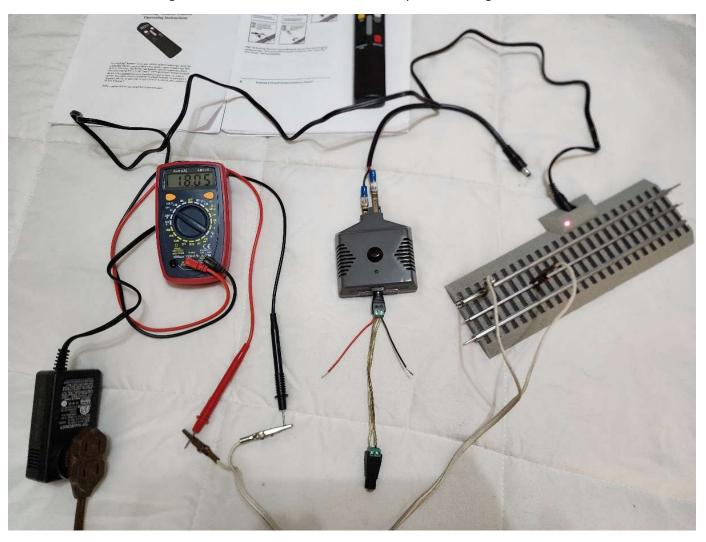
Moved meter to adapter, 2.1 mm x 5 mm, input to Lock-On shows 18 volts from Fast Track Transformer. Remote buttons have not been pressed. Adapter from Lock-On to Fast Track is 2.5 mm x 5.1 mm.
