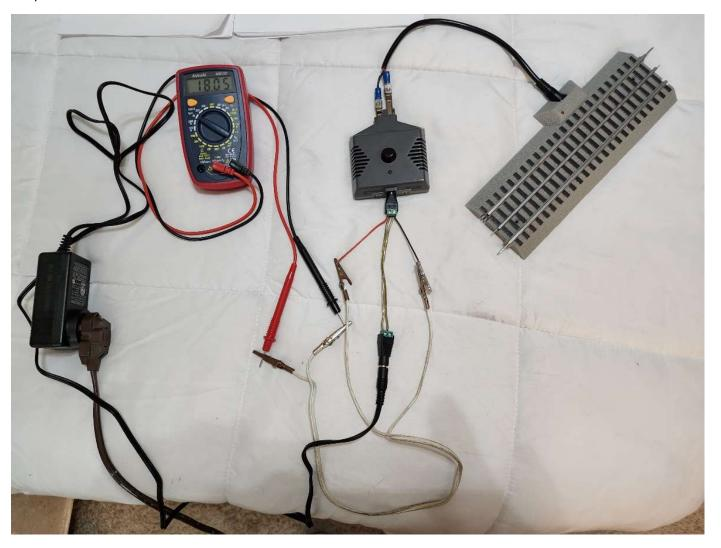
IR Lock-On connected to track, button on IR remote is being pressed, no green light on lock-on and no track voltage. Lock-On is not functional.
