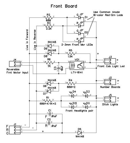
The R2LC/R4LC "ground" output is actually +ve (up to 9V half wave DC) and the lighting triacs are current drains back to ground. So the overall current flow in this diagram is CCW and all leds/diodes are oriented anode to the G terminal, cathode to the triac F & R drains. Since the lighting triacs operate on an either/or basis, led operation is determined by which one is active at any given time.
