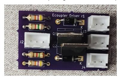
The circuit is quite simple: a PNP Darlington transistor current amplifier, powered from the DC supply full-wave bridge (FWB) rectifier and filter capacitor that powers the Blunami controller, often via a converter/regulator. Current capacity should be sufficient for any electrocoupler.
