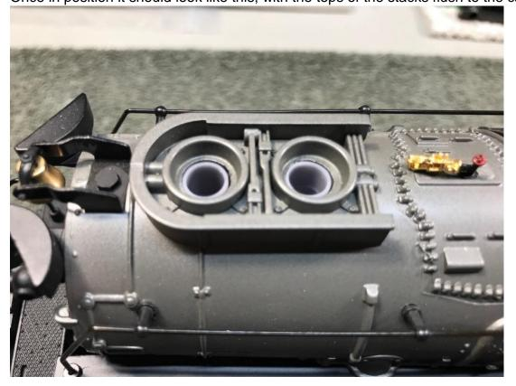
**Making It Puff:** Sadly TMCC pre-2004 engines with the 8057-200 smoke unit were not equipped to puff smoke, so you may wish to convert it at this time. (Later TMCC and Legacy with the 691-SSMU-F smoke units puff already) Your engine will look way more realistic with puffing smoke. This can be done using several methods as documented on the OGR forum. But the easiest method (as long as you are handy with wiring) is by installation of a JWA Super Chuffer, sold by Hennings Trains.
