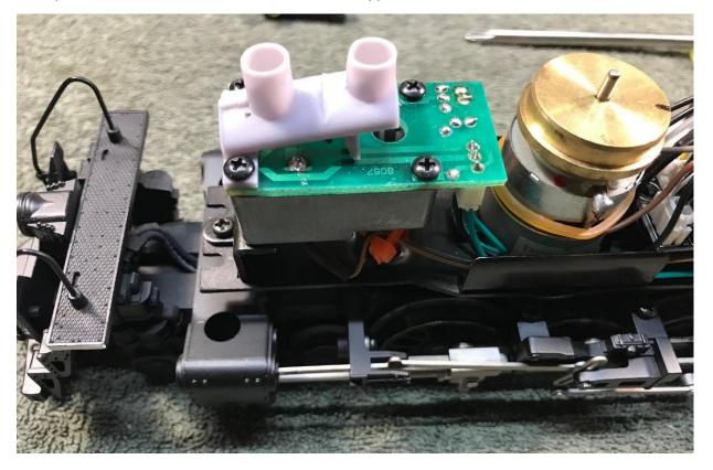
This picture shows the funnel mounted on a typical OEM 8057-200 smoke unit:
