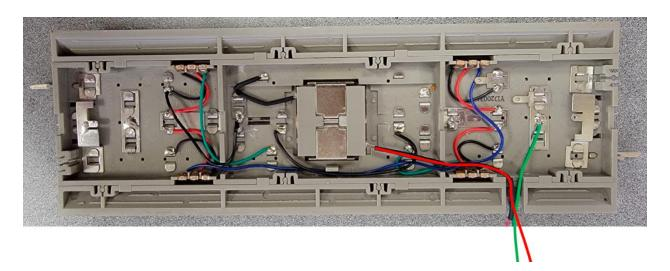
Step 6. Connect the accessory transformer PLUS/Hot to each of the other 2 momentary switches.
