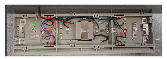
Step 5. Connect the 2 wires from the operation track section to one side of each momentary switch. One to the switch for UNCOUPLE and one to the switch for UNLOAD.
