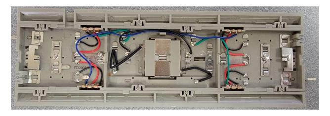
Step 2. Unsolder the electromagnet wire as circled below in yellow.
