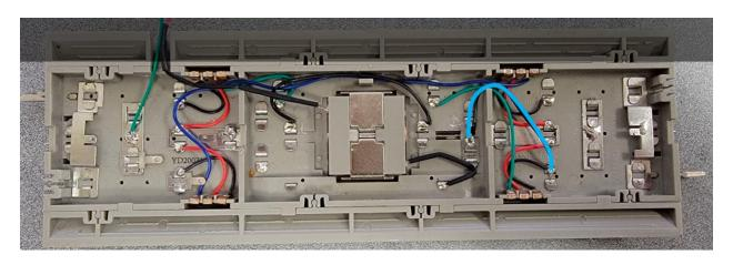
Step 4. Extend electromagnet wire that was unsoldered earlier (shown in red below). Also add a wire to the fifth-rail contact (shown in green below). Rung both wire to the outside of the track section as they will connect to the momentary switches on the layout control panel.
