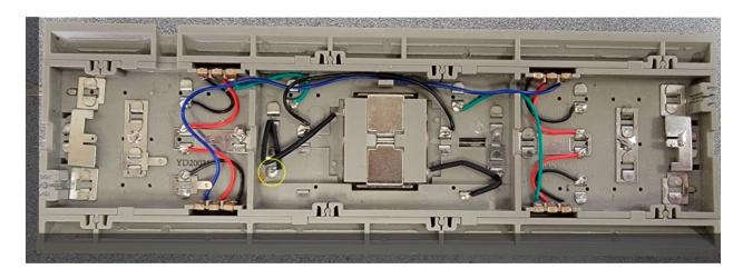
Step 3. Solder ground wire from where blue quick connect was to the adjoining outside reail as shown in light blue.
