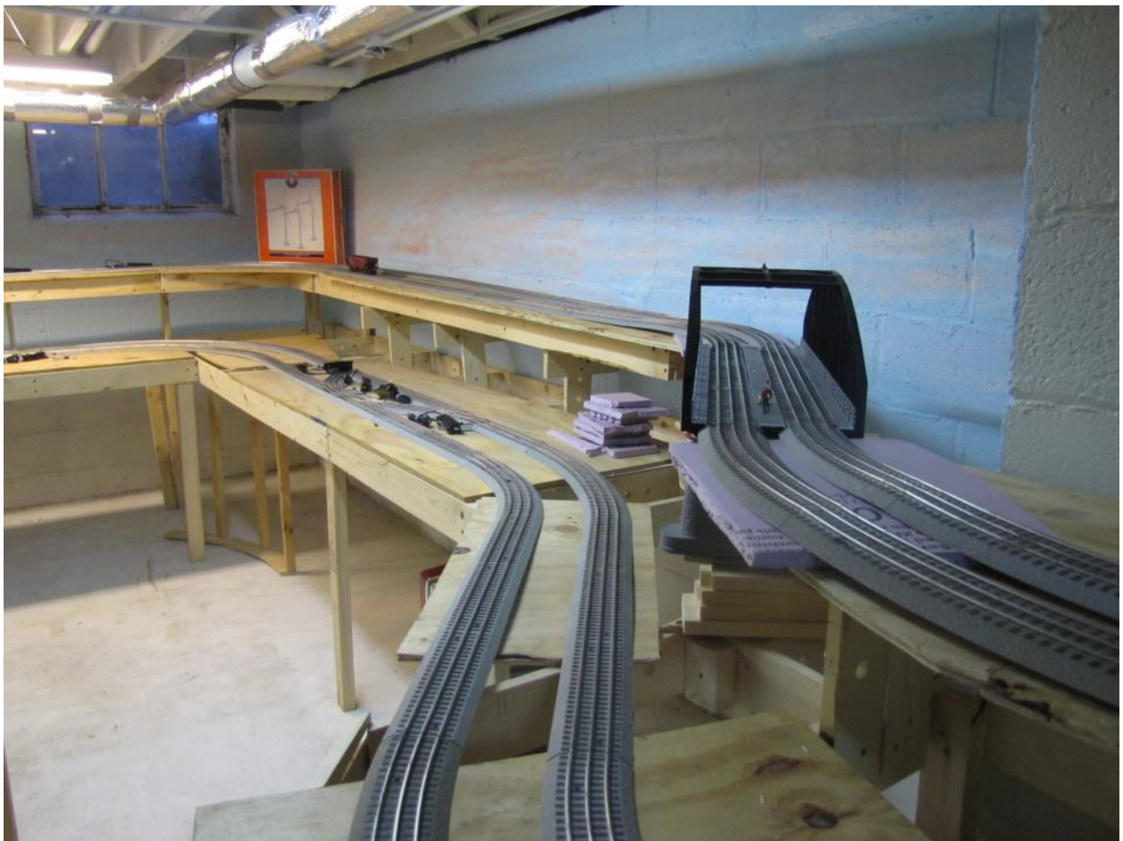
Facing Southeast: Low line (Left) and Highline (Right) Canyon/Bridge Approaches. (Note: Highline grade thru bridge approaches is 0%. Then continues upgrade to summit in far corner).
