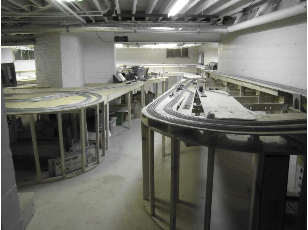
Facing East: Left: Eastern Division, Nested 0-60/-48; Center: Main Aisle; Right: Western Division, Nested 0-72/0-60, Grade 2.3% to Highline;
