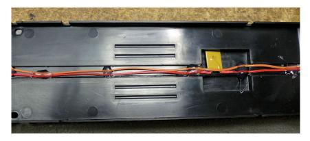
This is the completed lower level lighting. The connections for power come through the spring contacts on the left.
