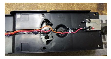
This is the middle of the car. Note the PTC to limit current between the rollers in the case of a derailment.
