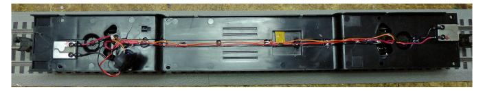
Here's the end of the car with the current conversion components completely assembled and the Velcro mounted for securing them inside the compartment
