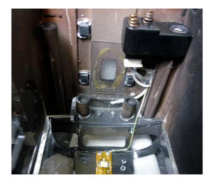
Two views of the detail of the current regulating module. The open wire hanging down is where the final wire will be connected, that's the constant current output. Note two regulators to support two LED strips.
