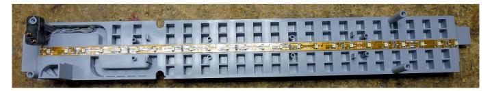
Here's the detail of the power connections of the lower level, they just tie into the existing connector for the spring contacts.
