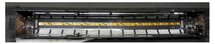
As with the lower level, the existing spring contacts are connected to the lighting strip and used to convey the power to the frame connection.
