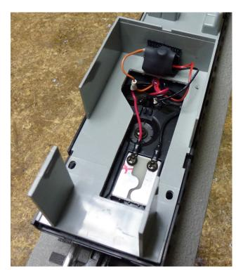
This is the completed top level lighting. As in the bottom level, the existing spring contacts are used to conduct power to the light strip.
