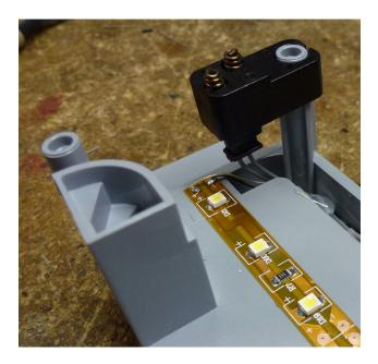
Here's the other end with the completed module attached with the Velcro to the bulkhead. The Velcro allows the module to be easily removed to lift the bottom seats off the chassis.
