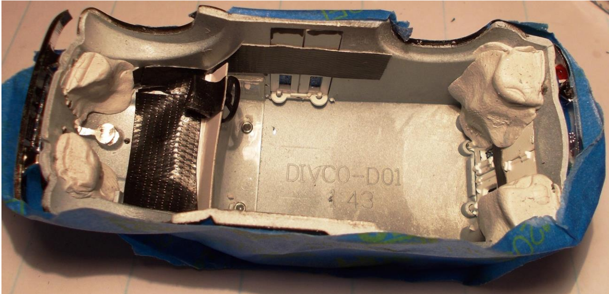
Figure 41: Four mounting-positioning towers were made from Repair Putty. Gorilla tape has been used to fasten doors somewhat better during modification (the 'Streets chassis will secure them firmly in place once inserted in body). Dashboard is just taped in place.
