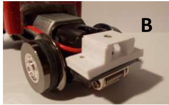
Figure 10: Scratch-built styrene trailer mounting platform is screwed on from beneath.
