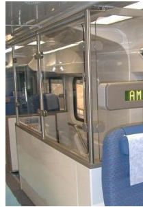
Upper Staircase Glass Partition
