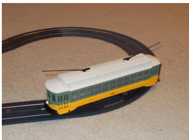
Figure 11: Most trolleys run through D-21 curves but only a few can handle D-16. This Atlas trolley runs well through D-16 but has had its truck swivel limiting screws removed, which required disassembly.
