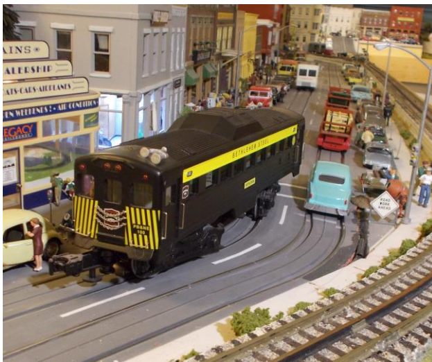
Figure 13: Just because you can...should you? This RMT Budd car (left) and Bang (right) will pass through the author's downtown loop. The BANG has been modified to increase its trucks' swivel angles so it will pass through D-16 curves as well as D-21. The Budd car is stock and makes it through D-21 and some D-16 curves, but only with great difficulty. While they both run on 'Streets curves, they are a hazard to everything around them as they do. On the left, the WBB sedan in the foreground is about to be knocked aside as the Budd car sweeps around the D-21 curve, and the BANG on the right side typically snags on a few parked cars unless they are moved well away from the edge of the 'Streets roadway's.
