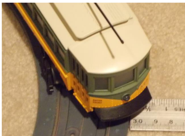
Figure 12: This Atlas trolley overhangs the outer edge of the road by about \frac{7}{16} inch on D-16 curves and overhangs in the inner edge of its lane by about \frac{1}{4} inch. Some trolleys overhang more. See also Chapter 4, Figure 2.
