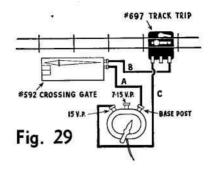
Connect wire "A" from one of the terminal posts on the Crossing Gate to the **base post** terminal on the transformer.
