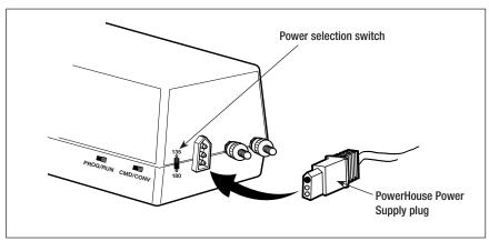
Figure 5. PowerMaster Installation
