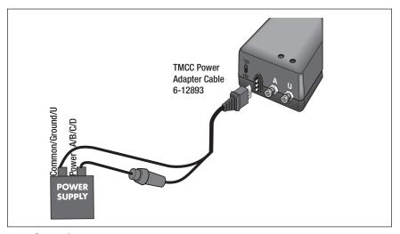
Figure 6. Transformer connection
