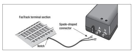
Figure 4. Transformer connections
