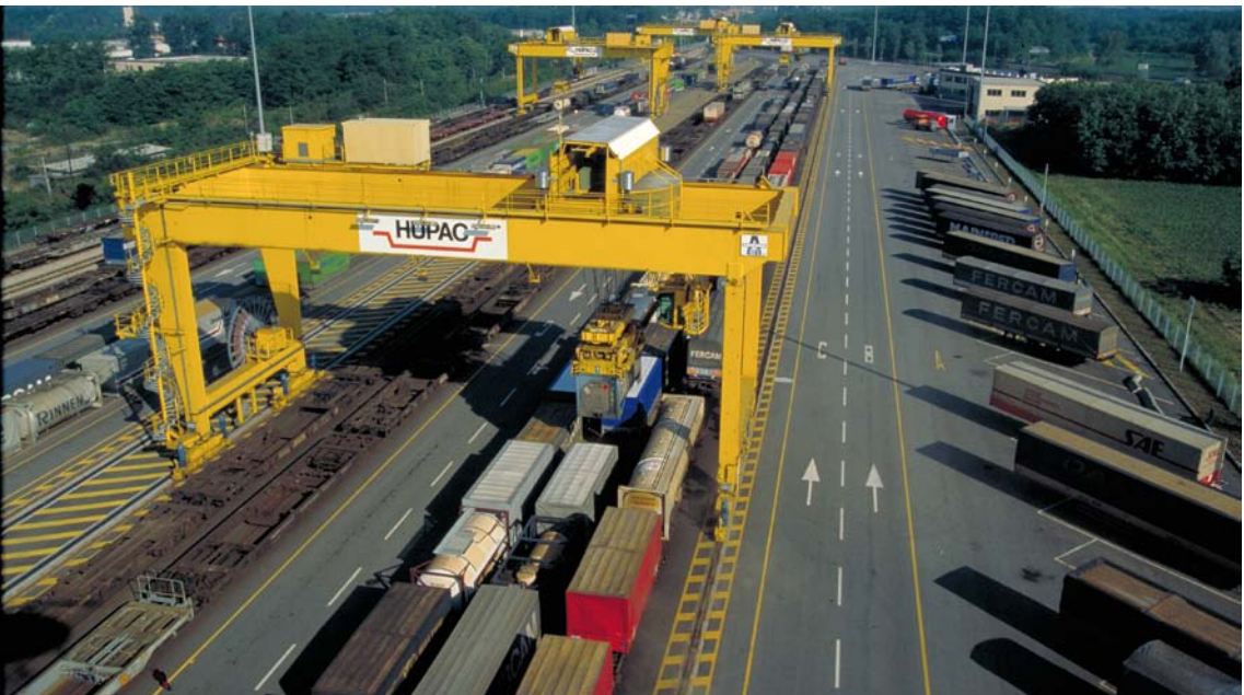
Right side of picture: Semi-trailers are prepared to be loaded on an intermodal train
