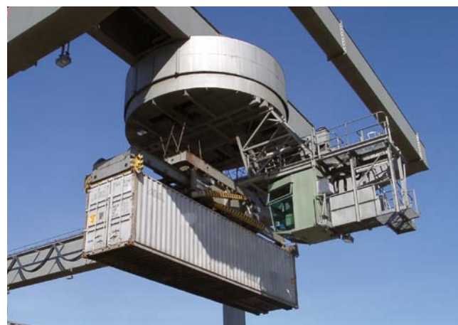
Crane turning the container by 180°
