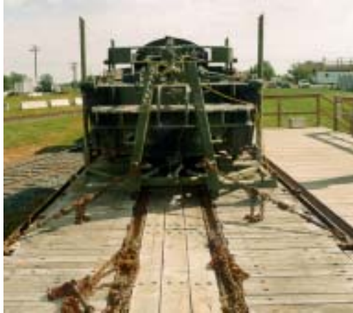
Figure 10. Chain Tiedowns on the Front of the IBC.
