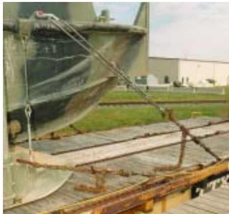
Figure 9. Chain Tiedowns on the Rear of the IBC and the Front of the Boat.
