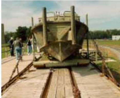
Figure 8. Chain Tiedowns on the Rear of the IBC and the Front of the Boat.
