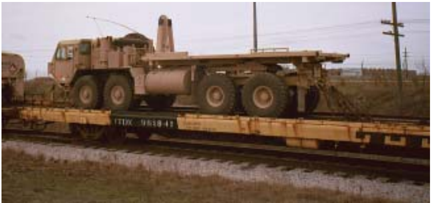
Figure 22. TTDX 89-foot flatcar; the deck layout is similar to the ITTX flatcar.
