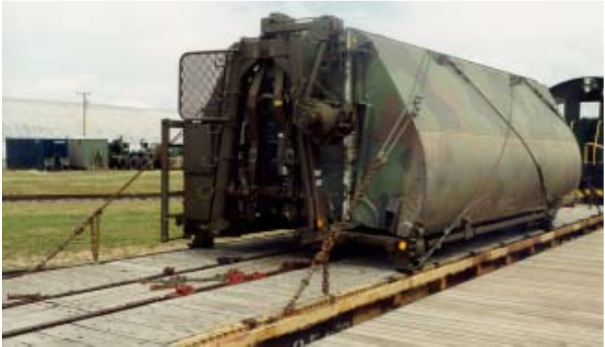
Figure 4. Side View of Tie-downs from Actual RIT.
