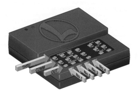
Connecting to SC-1. Middle-row terminals connect to common (ground) switch binding posts. Through and out connections connect to the upper and lower rows (respectively).
