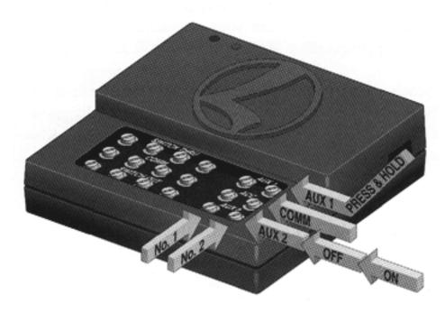
SC-1's accessory connections. The top row is for press-and-hold functions like loaders; bottom-row connections are for on-offs like floodlight towers. Use an SC-1 wallpack (no. AC160-1250) if your SC-1s controls accessories ONLY.
