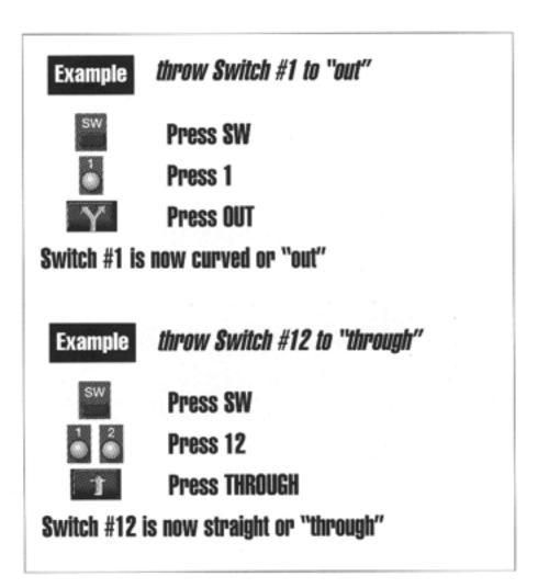
Now that you've programmed switch numbers, you can throw any SC-1-controlled switch using CAB-1.
