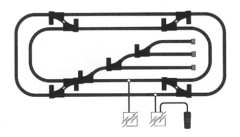
Now, install another power source, and you instantly divide your railroad's amperage load between two *blocks*. When you create blocks of electrical distribution, you can power *more* Command-equipped locomotives at once. Keep the size of the blocks small, and your Command-equipped Lionels will have all the power they need.
