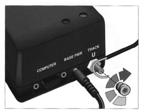
Connect a wire between the Command Base's binding post and the common (U) terminal on all PowerMasters or ZW transformers powering your track. You can also connect the wire between the Command Base and the outside rail of your track. (Connect the wire to both outside rails if you use hi-rail track.)
