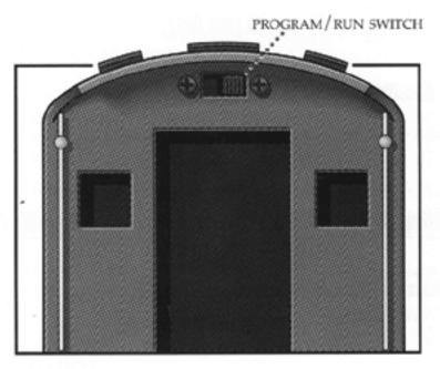
Slide the PROGRAM/RUN switch on your Command-equipped locomotive to PROGRAM. See your locomotive's owner's manual for the switch location and settings.
