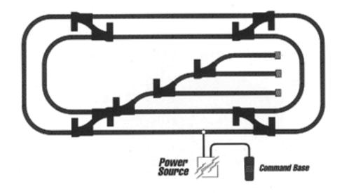
Here's a basic TrainMaster Command layout: two concentric loops linked by Lionel switches, with a small yard in the middle. If you're running only one or two locomotives at a time, this track plan will require only a single transformer for adequate power.
