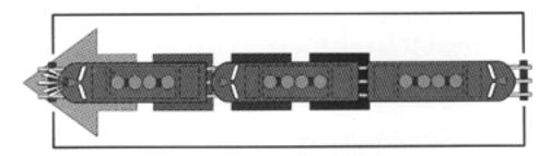
Pick the locomotives in your lash-up and move them together (but don't couple them) using ENG and each one's ID#. Because CAB-1's TR button also means "TRACK" for PowerMaster control, select a TRAIN (TR) ID# that is NOT a number identifying PowerMaster TRACKs. For example, if you're using four PowerMasters and have named their TRACKs 1, 2, 3, and 4, choose a number between 5 and 9 for your TRAIN ID#.
