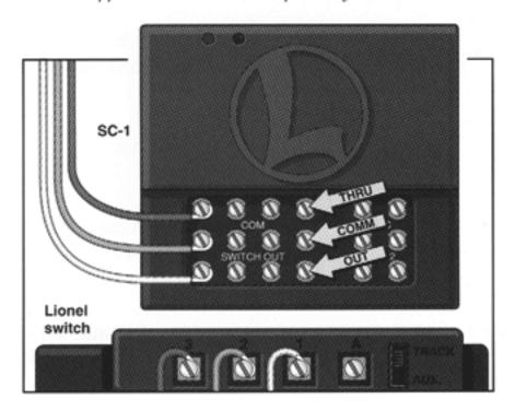
SC-1 ground (common) connections to popular Lionel switches. If your switch throws in the opposite direction, reverse the upper and lower terminal connections either on SC-1 or the switch itself.
