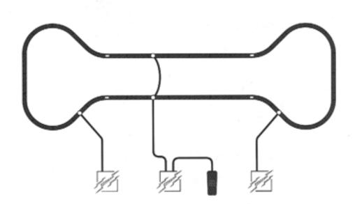
Add track and Command-equipped locomotives, and this giant of a model railroad needs two divisions. Just remember the formula: small blocks fed by healthy power sources. Your Command-equipped Lionels will give you superior performance when they have a dependable supply of power.
