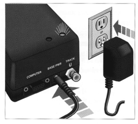
Plug the wallpack's cable into the Command Base power input, then plug the wallpack into a properly grounded wall outlet (110 volts, 50/60 cycles).
