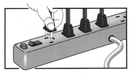
The easiest way to phase power supplies is by using a properly grounded power strip with circuit breaker.
