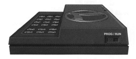
Slide SC-1's PROGRAM/RUN switch to PROGRAM. Using CAB-1, press SW, 1 on the numeric keypad, and SET under the removable panel. Slide the switch back to RUN. You're done.
