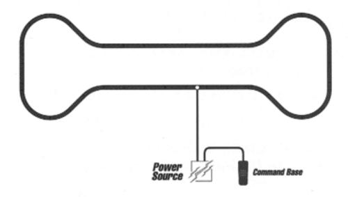
Multi-locomotive operation will cause a single power source to reach its limit quickly. Add electrically isolated blocks powered by healthy power sources, and your amperage worries are over.
