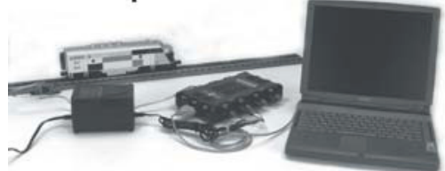
Computer Attaches To TIU RS-232 Port via a 9-Pin Serial Cable
