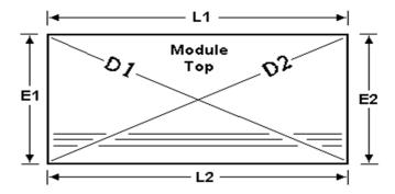
Lengths L1 & L2 should be equal, as should ends E1 & E2. Diagonal dimensions D1 & D2 should be the same.
