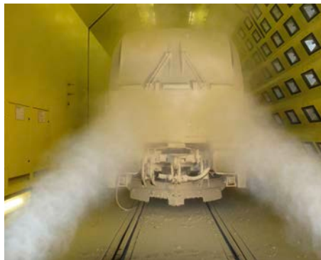
Vectron being tested in the Vienna Arsenal Climate Chamber
