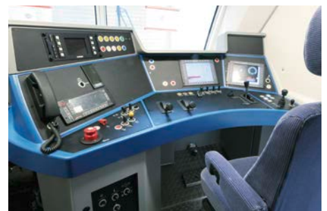
The driver's desk is also prepared for subsequent conversion or upgrading. Converting from high sun shades to low ones and vice versa is easily possible.
