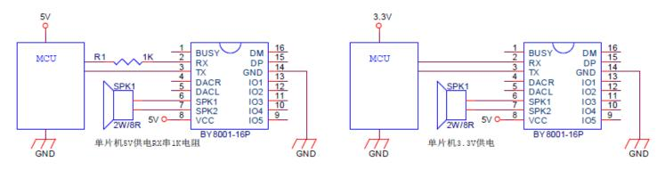
The above is a standard UART asynchronous serial connectivity applications, this application is quite flexible, including play, pause, down song, volume addition and subtraction, playing selections, wide Advertisement spots and so on. Available microcontrollers, computer serial port control 485 can also be controlled by TTL to RS485 adapter plate.
