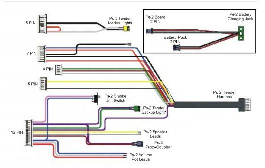
\*Note: If tender has harness to connect an auxillary tender, connect the back-up light and coupler connectors to the harness. Use switch to select light/coupler operation in tender or auxillary tender.
