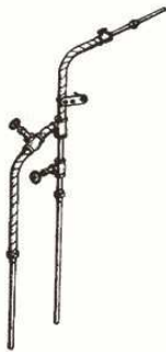
PSDR-1114 Pipes w/valves, cab left side, K-37
