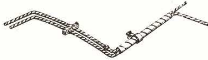
PSH-40424 NYC J3A Worthington feed water heater steam supply plumbing fireman's side
