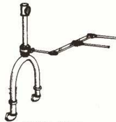
PSCC-7017 Steam pipe, turret & throttle, 18 ton Climax
