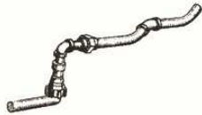
PSH-40330 Fireman's side plumbing, under cab mount, Niagara
