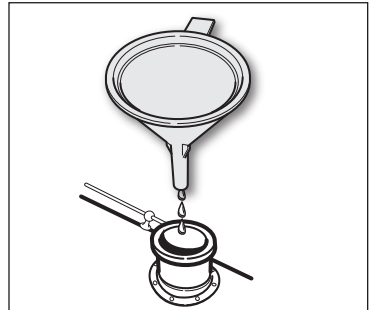
Figure 1. Adding smoke fluid to the main stack
