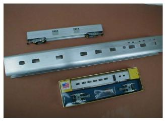
"Pennsy" style smoothside siding available in HO and O gauge. This siding is completely smooth from roof to wheel skirts. Available only through our custom car
